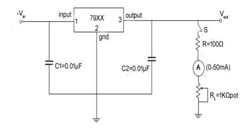
Figure: 3. Negative Voltage Regulator
