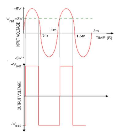
Fig. (a) When  $V_{ref} = 3V$
