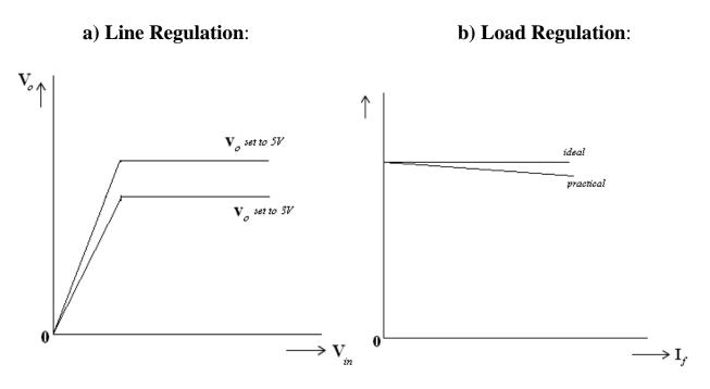
**Results:** Low voltage variable Regulator of 2V to 7V using IC 723, 7805, 7809.7912 is Designed. Load and Line Regulation characteristics are plotted.
